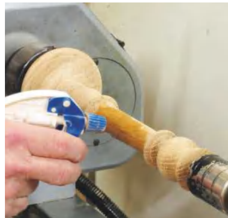
▲ Pic.30 The second candlestick is going to have the paint effect on it. Firstly, wet the timber with water from an atomiser bottle; this will slow down the burning process
